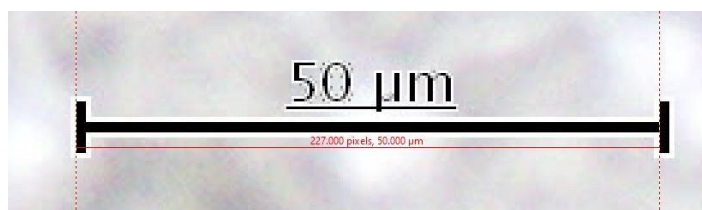
Figure 4: Image of calibrating protocol, aligning 50 µm scale bar and related pixel count using ToupView software.
