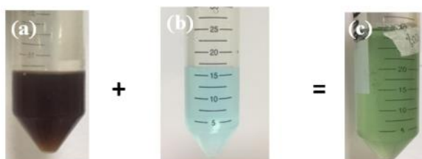
Figure 2b: Color reaction of the formation of green synthesized copper oxide nanoparticles, (a) C. cujete leaves extract; (b) copper salt, (c) CuONP from C. cujete
